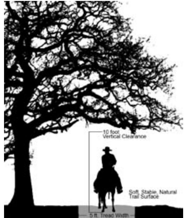
Figure 2: Equestrian Trail Clearance Requirements
