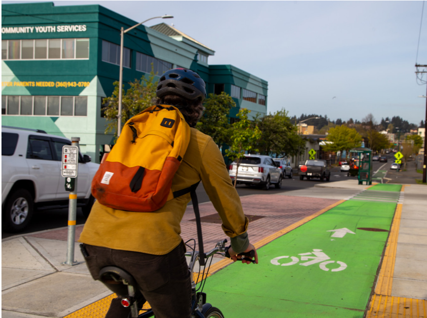
▲ Photo: Enhanced separated bike lane near the intersection of State Avenue NE and Plum Street Southeast. [City of Olympia]
