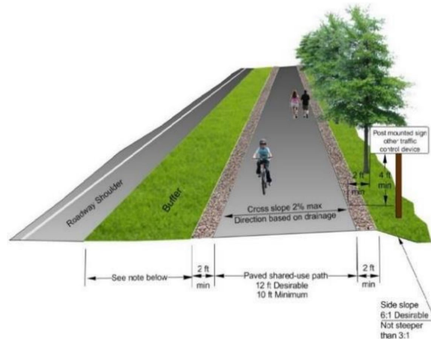
Figure from the WSDOT Design Manual, Chapter 1515. Buffer must be at least 3 feet for roadways \geq 35 mph and greater than 5 feet for roadways > 35 mph.
