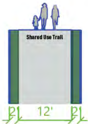
Figure 18. Shared Use Trail Cross-Section
